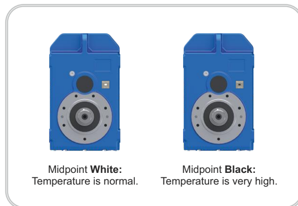
Figure 9: Temperature Sticker (M)
