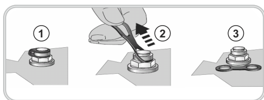
Figure 5: Activation of Vent Plug
