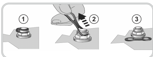
Figure 3: Activation of Vent Plug
